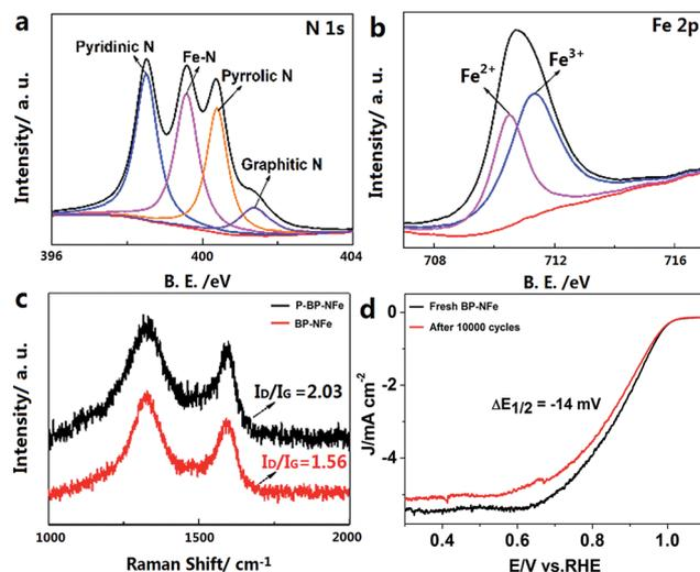
Fig. 4 High-resolution XPS spectra of N 1s (a) and Fe 2p (b) of the BP-NFe catalyst. (c) Raman spectra of the P-BP-NFe and the BP-NFe catalysts. (d) The durability of BP-NFe in O<sub>2</sub>-saturated 0.1 M KOH.
