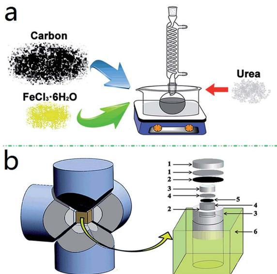
**Fig. 1** Scheme of UHP synthesis: (a) precursor processing and (b) UHP synthesis at controllable high temperature and the schematic diagram of the pressure cavity in the cubic anvil high-pressure apparatus, and the assembled chamber ((1)-steel plate, (2)-graphite heater, (3)-dolo-mitic cylinder, (4)-molybdenum box, (5)-sample, and (6)-pyrophyllite).
