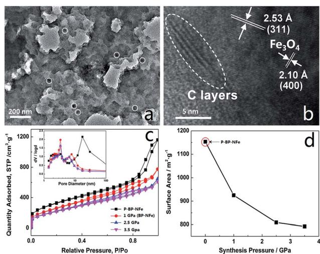
Fig. 3 (a) TEM and (b) HRTEM images of BP-NFe. The white circles indicate the distribution of Fe nanoparticles in (a). (c) Nitrogen adsorption-desorption isotherms, the inset is pore-size distributions; (d) synthesis pressure dependence of the Brunauer-Emmett-Teller (BET) surface area.
