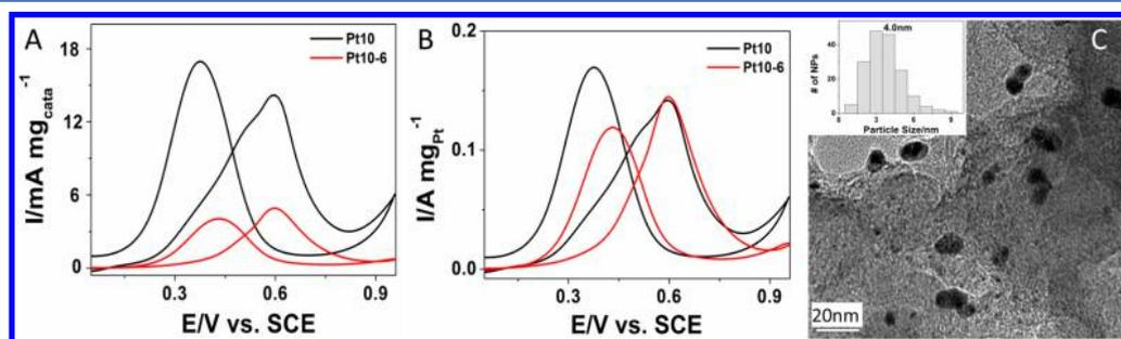
**Figure 4.** Effect of the “regeneration process” with additional carbon on the fresh Pt/C (Pt10): (A) decrease in the apparent activity (mA mg<sub>cata</sub><sup>-1</sup>) after the treatment; (B) there is no improvement of Pt utilization (A mg<sub>Pt</sub><sup>-1</sup>) after the regeneration process; (C) typical TEM image and the size distribution of Pt after the regeneration process.
