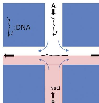
**Fig. 1** The scheme for single molecule experiments with stagnation point flow, arrows show the flow directions in the cross-slot device. Individual DNA molecules flow in from channel A where they are trapped and stretched at the stagnation point. If there is extra NaCl flowing in from the opposite channel B, Na<sup>+</sup> will combine with the DNA molecule and induce its compaction which can be monitored by fluorescence microscopy.
